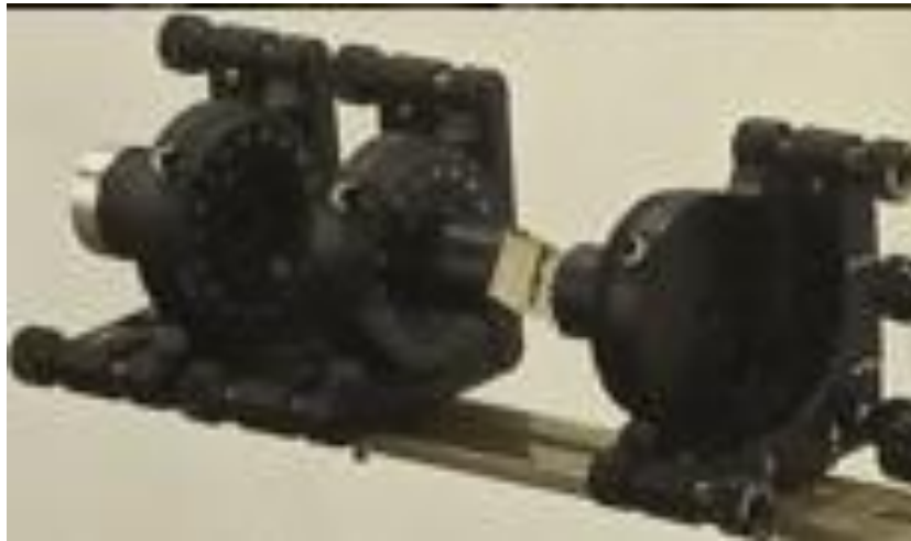
Figure 2. 4 CSP (consisting of retarder R_1 , retarder R_2 , and analyzer A )
